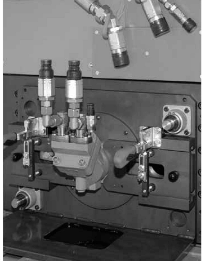
test bench for motors
