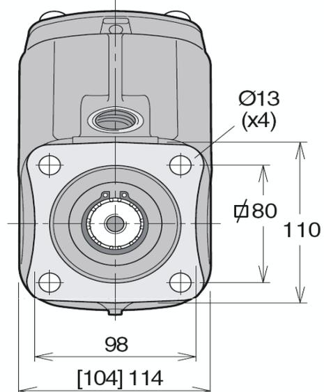
**Note ! Drain line must be mounted. Connection BSP 1/2". Maximum drain line pressure is 3 bar**
