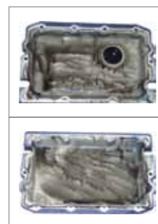
CH-4 Chemistry 81.000 Km/50.000 mile oil drains
