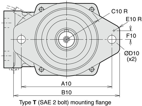
Type T (SAE 2 bolt) mounting flange
