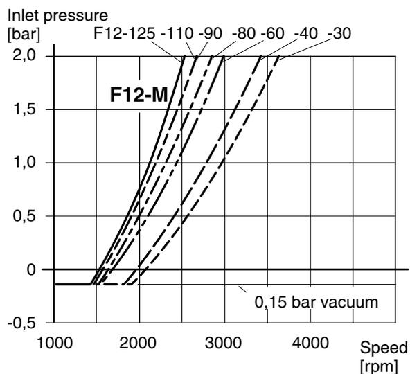
Diagram 3. Min. required motor (F12-M) inlet pressure.
