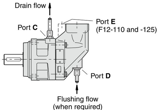
In mounting positions such as 'shaft up' (below) a spring loaded check valve should be installed in the drain line in order to insure a sufficiently high oil level in the case.
