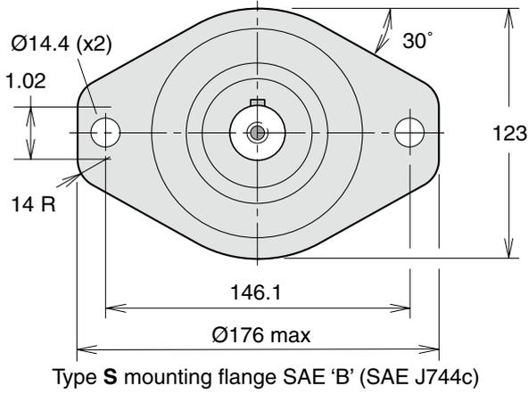
Type S mounting flange SAE 'B' (SAE J744c)
