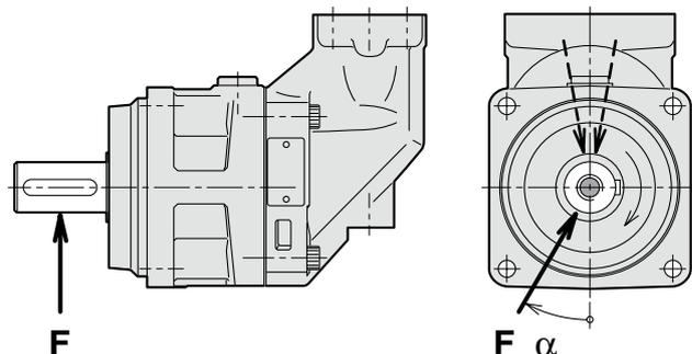
The direction (a) of the radial load is positive in the direction of rotation as shown.
