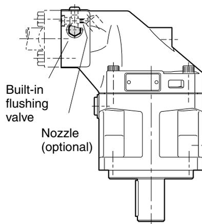
Integrated flushing valve (F12-30, -40, -60, -80, -90) Nozzle (optional)
